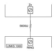
LINKS circuit board. The zone programmed as LINKS Answer always requires a single EOL resistor ( $5600\Omega$ ).
